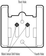
3. Continue to hold the bracket on the transom of the boat, and use a pencil or marker to mark where to drill the two mounting holes. Mark the drill holes near the top of each slot, making sure that your mark is centered in the slot.
